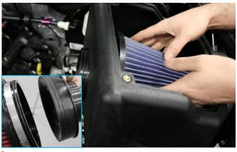
8. Install filter adapter onto Volant air filter, then place air filter into Volant air box.
