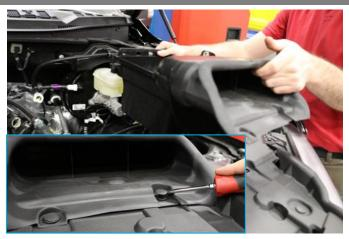
Remove the two clips holding the factory scoop using a pry tool. Save clips for Install Step 5. Remove scoop and air box assembly from vehicle.
