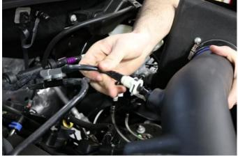
13. Connect factory quick disconnect to the Volant air duct.
