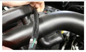
2. Release the coolant hose from the factory air duct.
