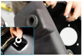
2. Put the metal bushing and rubber grommet from **Removal Step 9** into the Volant air box.
