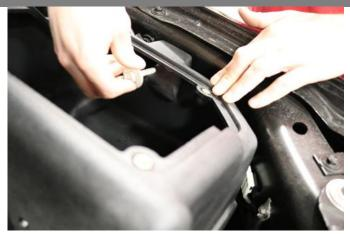
Use the bolt saved from Removal Step 7 to attach the Volant air box to the fender with a 13mm socket.
