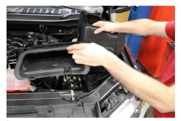
4. Install the factory air scoop, and Volant air box into vehicle making sure to place the studs on the bottom of the air box into factory grommets.
