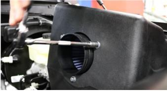
9. Secure the filter adapter to the Volant air box using a 10mm socket and three M6-16mm bolts, lock washers, and flat washers.
