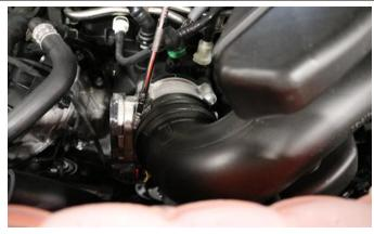
1. Loosen the throttle body clamp using a 7mm socket.
