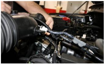
3. Disconnect vent connection from the rear of the factory duct.
