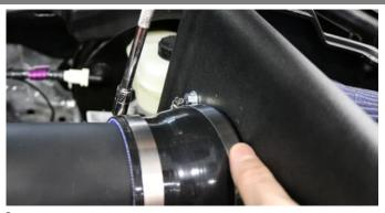
12. Insert the air duct onto the straight sleeve on the throttle body and large end of reducer onto the filter adapter. Adjust Volant air duct to proper fit and tighten all clamps using an 8mm socket or flat head screwdriver. NOTE: Also tighten the filter's clamp at this time.
