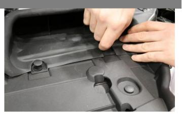
Re-install the factory scoop with clips saved from Removal Step 8.
