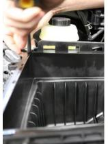
6. Use a pry tool to remove the three wire retention clips.
