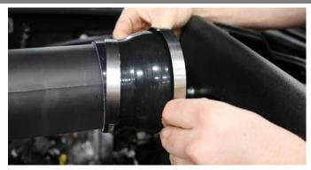
11.Install one #56 clamp on small end of the reducer, and one #64 clamp on larger end of reducer. Place small end of reducer onto straight end of Volant air duct.
