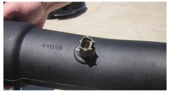
Locate air temperature sensor from removal step 9 and Volant air duct. Install sensor into grommet with tab facing the closest end of air duct.
