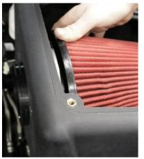
9. Insert the filter into the air box with the adapter side down. Rotate the top of the filter down into the air box and rotate the filter around and push the adapter through air box.
