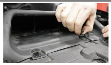
Reinstall factory scoop and attach with clips from Removal Step 6.
