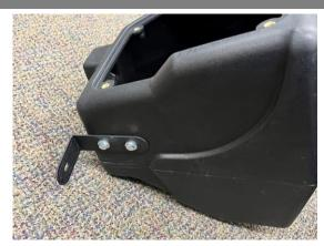
1. Install wiring harness bracket to Volant air box using two 6mm x 16 bolts, two .25" x .63" flat washers, two .25" lock washers and two 6mm nuts.
