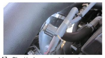
17. Clip wiring harness on air temperature sensor.
