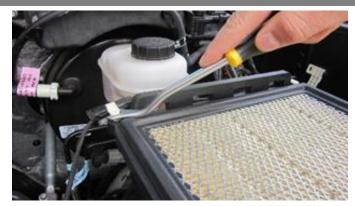
5. Remove the three plastic wire retention clips from back of factory air box
