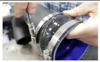
12. Install the hump hose onto the Volant air duct along with two #64 clamps and tighten using a ratchet and 8mm socket or flat head screwdriver. Leave clamp on open end of hump hose loose.
