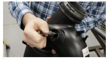
Remove the air temp sensor from factory duct. Save for Install Step 17.
