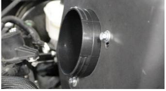
Locate three 6mm x 16mm bolts, three .25" x .63" flat washers, and three .25" lock washers.
