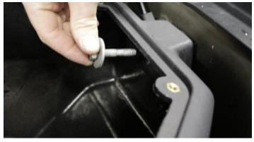
5. Attach the Volant air box to the fender with the bolt from **Removal Step 4** using a ratchet and 13mm socket.
