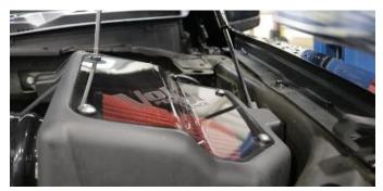
Install lid using provided 4 truss head screws with rubber washers and Philips head screwdriver.
