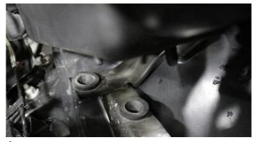
Install Volant air box into the vehicle by inserting stems on bottom of Volant air box into factory grommets.
