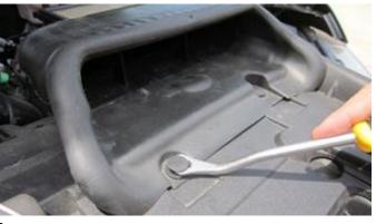
6. Remove the two plastic clips from the factory air scoop. Save clips for **Install Step 7**.
