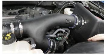
16. Adjust air duct as necessary and tighten all clamps using a ratchet and 8mm socket or flat head screw driver. NOTE: Make sure to tighten the filter clamp as well.
