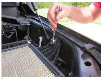
4. Use a ratchet and 13mm socket or wrench to remove the bolt holding the air box to the vehicle. Save bolt for **Install Step 5**.
