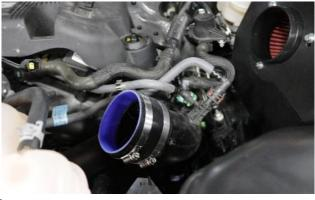
13. Install the straight sleeve onto lower factory inlet with #64 clamp. Tighten clamp using a ratchet and 8mm socket or flat head screwdriver. Leave clamp on open end of straight sleeve loose.
