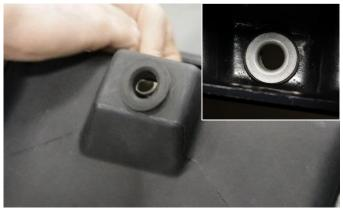
Insert the factory grommet from Removal Step
