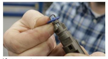
10. Remove O-ring from the temp sensor.
