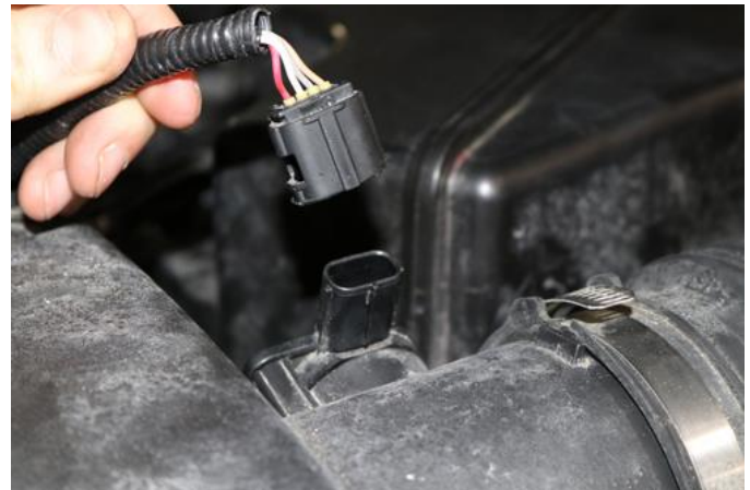
4. Disconnect MAF sensor.
