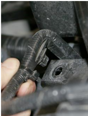
3. Undo two MAF sensor wire retaining clips.
