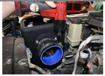
5. Install the hump hose onto the Volant filter adapter along with a #56 clamp. Tighten the clamp using an 8mm socket or nut driver.
