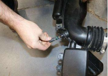
10.Remove ATS from factory air duct by gently lifting tab and twisting.
