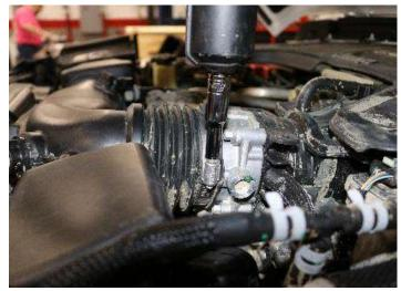
7. Loosen clamp holding factory air duct to throttle body using an 8mm socket and ratchet or flat head screwdriver.
