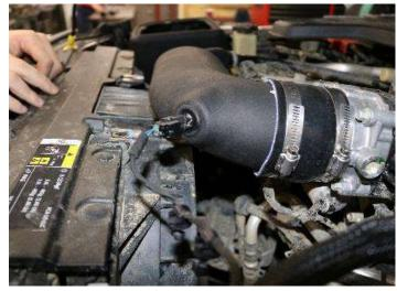
11. Reconnect the factory air temperature sensor wiring harness to the sensor.
