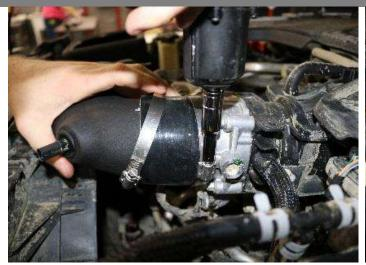
9. Tighten the clamp holding the straight sleeve to the throttle body with an 8mm socket or nut driver, ensuring the straight sleeve is completely bottomed out. Tighten the remaining clamps, taking care that the Volant air duct has clearance above the fan shroud.
