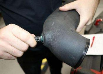
2. Press the air temperature sensor into the grommet in the Volant air duct. A light amount lubricant will help installation.
