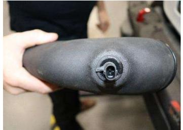
3. Make sure the sensor is oriented as shown.
