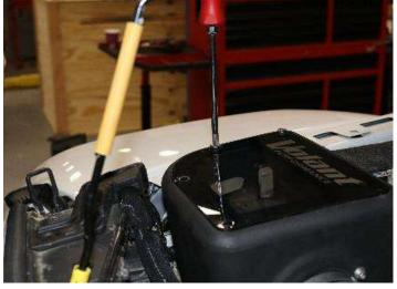
16. Secure lid to Volant air box with the (5) provided truss head screws and rubber washers, using a Philips head screwdriver. Tighten only enough to slightly compress the lid gasket..
