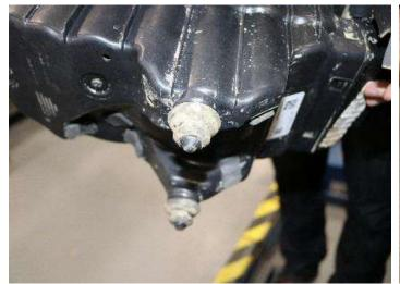
9. Remove both grommets from bottom of factory air box. Save for reinstallation.
