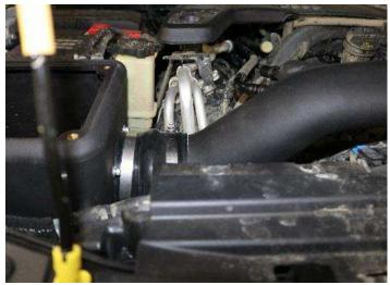
Install Volant air duct into hump hose along with a #56 clamp. Do not tighten the clamp at this time.
