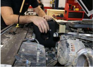
4. Place the Volant air box into the vehicle by fitting the bottom of the box into the (2) grommets from install step 1.
