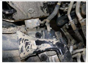
1. Place the (2) rubber grommets from removal step 9 back into the factory location.
