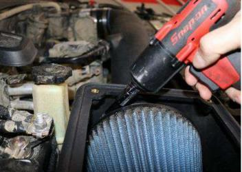
14. Tighten the filter clamp using an 8mm socket or nutdriver.
