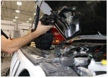
8. Remove factory intake as one assembly by pulling up, then out. Save in case vehicle needs to be returned to stock.
