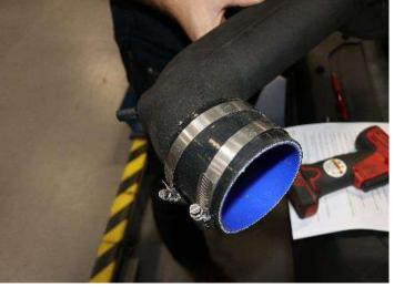
6. Install the straight sleeve onto the shorter end of the Volant air duct along with a #56 clamp. Do not tighten clamp at this time.
