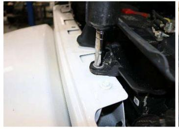
5. Remove the 10mm bolt holding the factory air box to the fender using a 10mm socket and ratchet. **Save for reinstallation.**
