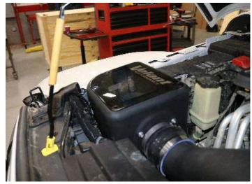
15. Install the Volant lid onto the Volant air box.
