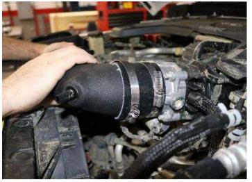
8. Install the straight sleeve onto the throttle body along with a #56 clamp. Do not tighten clamp at this time.
