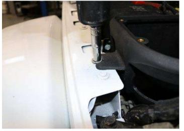
12. Secure Volant air box to the fender with the bolt from removal step 4 and included washer, using a 10mm socket.
