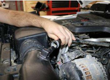
6. Disconnect the breather hose from the factory air duct.
