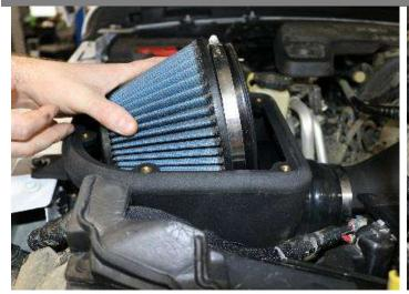
13. Install the Pro5 Filter #5120 or PowerCore Filter #61513 along with clamp into the Volant air box and onto the filter adapter. Make sure to press the filter onto the adapter completely so it is bottomed out.
