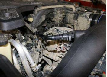
10. Reconnect the factory breather hose to the fitting installed in the Volant air duct.
