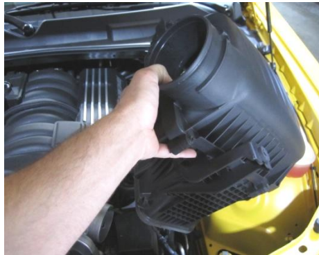
Remove the factory air box and duct.
