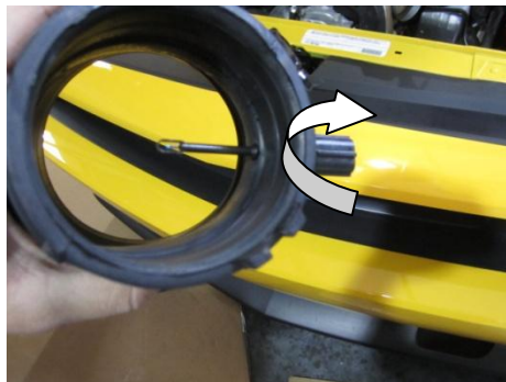
Remove the factory ATS by twisting and pulling up and out.
