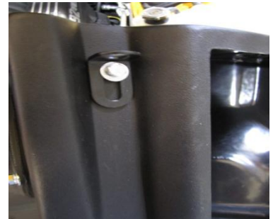
Install the supplied bracket to the volant box using the supplied hardware.
