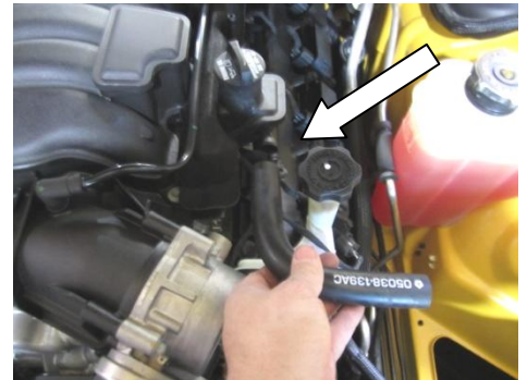
Remove the factory breather hose.
