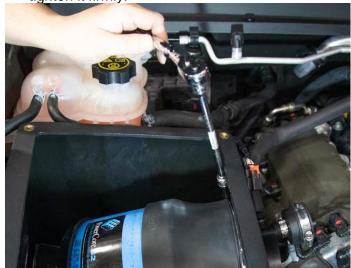
7. Insert the filter into the airbox and place it over the filter adapter. Tighten the filter clamp securely using an 8mm socket and ratchet.
