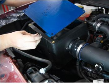
15. Remove the protective blue film and then place the Volant lid over the airbox and secure it using the lid screws provided. Tighten the lid screws using a Philips head screwdriver. DO NOT overtighten.
