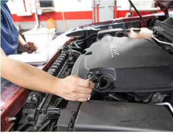
6. Remove the engine oil cap.
