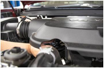
4. Unclip the vent line fitting by pressing on the side and pulling it gently.
