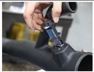
1. Insert the MAF sensor into the duct as shown with the MAF sensor gasket provided sandwiched between the MAF and the Duct.
