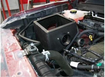
4. Carefully place the Volant airbox as shown making sure to insert the fitting at the bottom of the airbox into the grommet in the engine bay.
