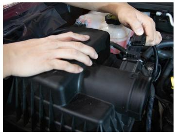
Unclip the factory MAF sensor harness by pulling on the tab till it clicks and then pressing it and pulling it as the same time.
