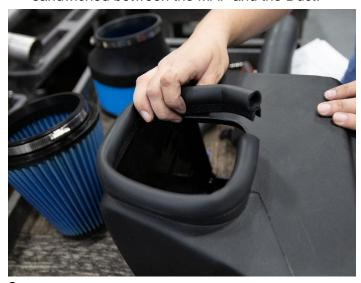
3. Insert the provided Bulb Seal to the Volant airbox as shown.
