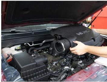
7. Carefully lift the engine cover along with the factory airduct and place it aside.
