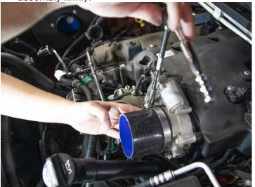
8. Insert the provided straight sleeve over the throttle body along with a 3" clamp as shown and secure the clamp using an 8mm socket and ratchet.
