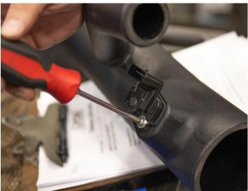
2. Use the two Philips head screws and screw the MAF sensor to the duct securely.
