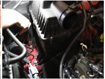
Using a 10mm socket and a ratchet with extension, remove the 2 nuts shown above. Keep 1 nut for use with installing your Volant Intake
