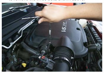
3. Loosen the clamp shown above using an 8mm socket and ratchet.
