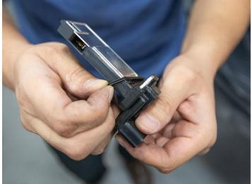
12. Remove the factory MAF sensor gasket shown above and place it aside. Keep the MAF sensor for use with the Volant Air Intake.
