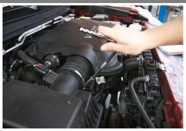
2. Loosen the duct clamp shown above using an 8mm socket and ratchet.
