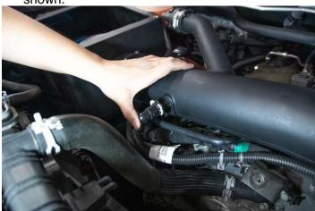
12. Insert the factory vent line into the duct fitting by pushing it firmly until it clicks.
