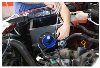
9. Insert the provided hump hose into the filter adapter along with a 3.5" clamp and secure the clamp using an 8mm socket and ratchet.
