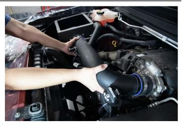
10. Insert the duct into the straight sleeve on the throttle body and the hump hose on the airbox as shown.
