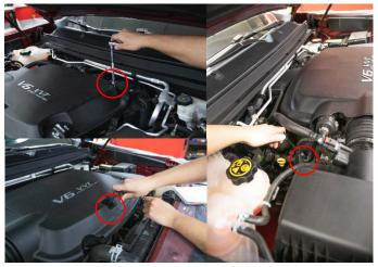
1. Use a 10mm socket and ratchet with extension to remove the three bolts shown above.
