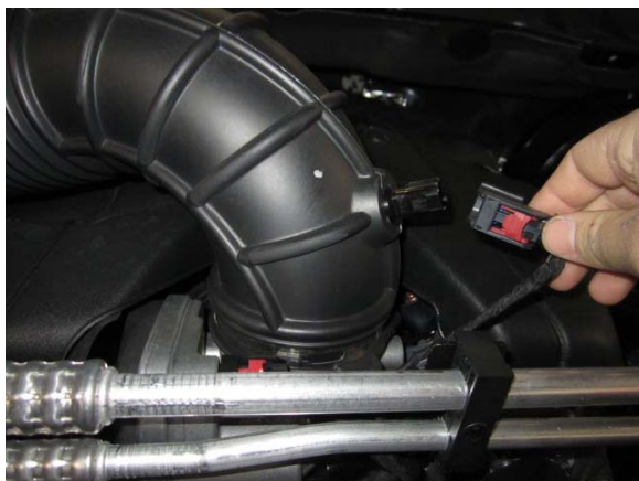
1. Disconnect air temp sensor on the air duct.
