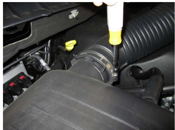
2. Loosen the hose clamps on the air duct located on the filter box and throttle body and remove the air duct.
