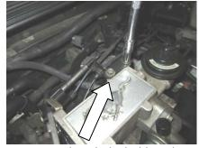
6. Remove the 2 bolts holding the throttle cables in place.
