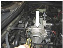
4. Remove the 4 bolts holding the throttle body in place.
