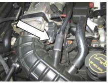
9. Reattach the factory air duct and breather hoses. Use the 5/8 breather hose to connect the factory hard line to the fitting installed in step #8.
