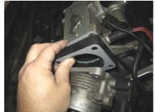
7. Place a gasket on each side of the spacer and install with the curved edge of the fins facing the throttle body.
