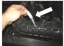
8. Place the 5/8 fitting into the factory air duct nearest the throttle body.
