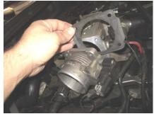
5. Remove the factory throttle body gasket.
