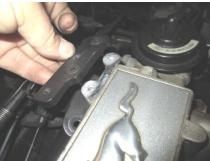
10. Install the cable extension bracket into the factory location using the supplied allen screws.
