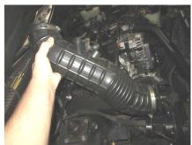
3. Remove the factory air duct.
