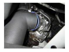
16. Attach the air duct to the reducer using the #48 clamp
