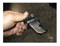
12. Replace the factory sensor gasket with the supplied Volant gasket.
