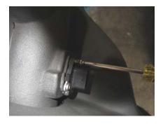
13. Attach the MAF sensor to the Volant air duct.
