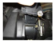
11. Using the T-20 Torx bit remove the factory MAF sensor.
