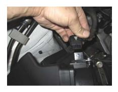
3. Disconnect the MAF sensor harness from the MAF sensor.
