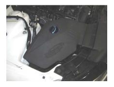
15. Press the Volant box into the factory rubber grommets and into the factory scoop.
