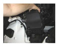
5. Remove the factory air box by pulling up and out.
