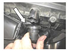
Disconnect the vent pipe from the factory <u>air box</u>.
