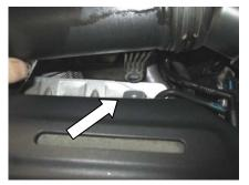
Remove the screw holding the duct to the engine.
