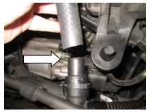
Press the 1" hose onto the adapter.
