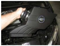
Install the Volant air box onto the factory studs and attach the supplied hump hose.
