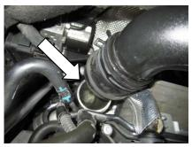
Loosen the clamp holding the air duct in place and lift up on the air duct.
