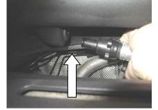
Press the hose adapter into the vent hose until it clicks and press into the rubber grommet.
