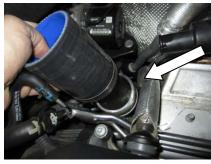
Attach the straight sleeve onto the engine using the provided clamp.
