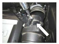
Remove the factory MAF sensor.
