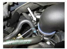
Press the Volant air duct into the hump hose and sleeve. Tighten the clamp holding the sleeve to the duct.
