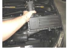
Remove the factory air box by pulling up and releasing it from the factory rubber grommets.
