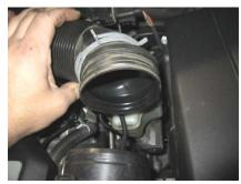
Remove the factory air duct from the factory MAF adapter.
