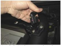
Attach the MAF sensor to the Volant duct using the self tapping screws and MAF gasket. Reattach the negative battery cable.
