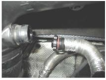
Disconnect the vent pipe from the air duct.
