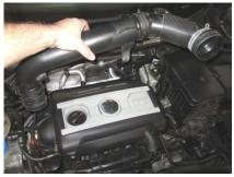
Remove the factory air duct.
