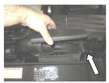
Remove the factory air inlet cap.
