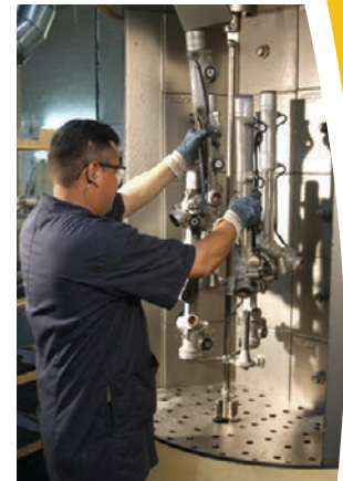
Shot-blasting rack and pinion housings removes dirt/rust and renews the appearance to "like new"
