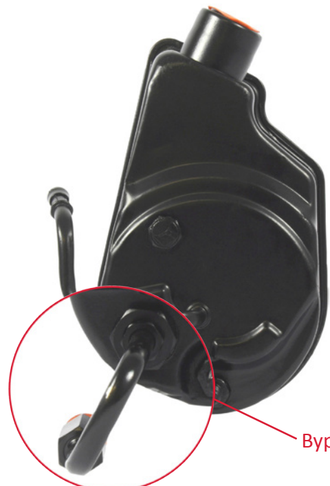
Pump with Bypass Pipe Installed
