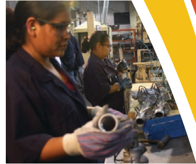
Gauging of parts to check critical dimensions
