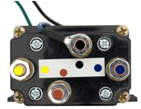
Connect BLUE post to the winch BLUE post Connect YELLOW post to the winch YELLOW post Connect RED post to the battery POSITIVE post Connect BLACK post to the battery NEGATIVE post
