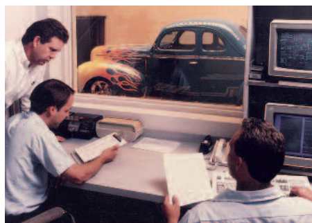
Re-engineering Our Systems To Perform Well With The 134a Refrigerant Required Many Months Of R&D. This Photo Shows Some Of The Testing For These New Systems.
