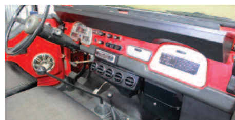
U.S. spec Toyota FJ-40 Land Cruiser dash using factory controls and Vintage Air louvers.
