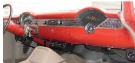
1955-56 Chevy installation with center plenum.
