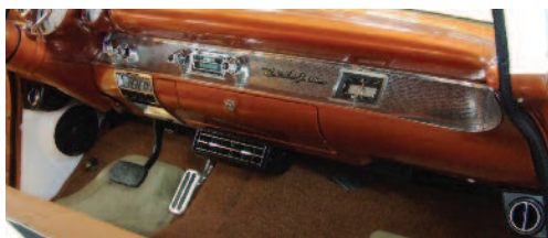
1957 Chevy installation with center plenum.
