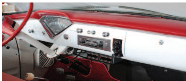
1955-59 Chevy Truck dash with SureFit kit and standard rotary replacement control panel.
