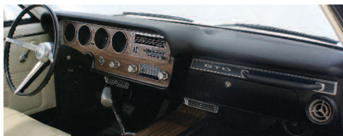
1966 GTO factory-air dash with SureFit kit. (Note: SureFit installations in factory air equipped GTO use the original in-dash A/C louvers.)
