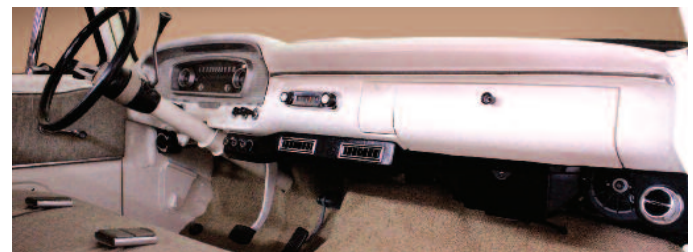
1961-66 under dash panel and louver package shown.
