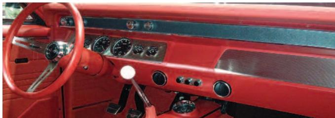
491210-RUA Gen IV 3-Knob Controls (Installed into a custom console), and 499194 Double Vane Louvers
