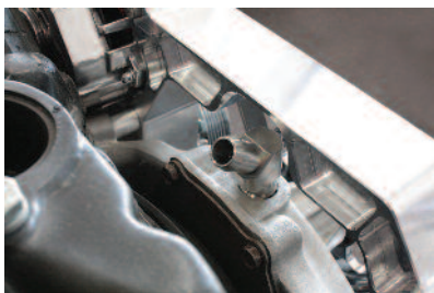
OEM-Style Water Pump Bypass Design
