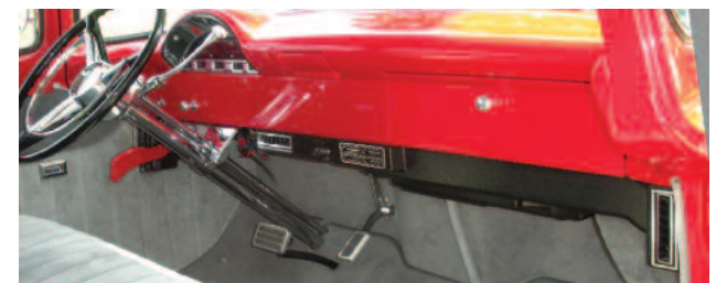
Under dash panel with louver package shown is available with or without control panel installed.
