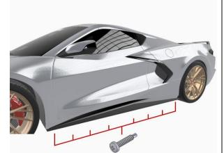
(1) Align splitter w/ rocker panel & proceed to install side splitter using self-drilling screws or hardware of your preference
