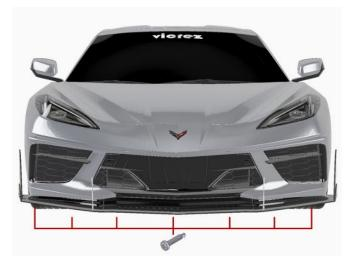
(2) Align the splitter w/ bumper & proceed to install front splitter using drilling screws or existing OEM hardware
