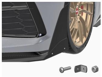
(1) Install the winglets with the hardware provide (screws, nuts, & brackets)
