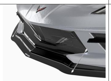
(3) Support rods can be installed in any placement of the bumper. However, it is not required for installation
