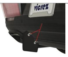
(4) Align the fins accordingly, mark holes & proceed drilling fins for the bracket, use self-tapping screws to attach fins to OEM rear diffuser
