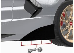
(2) After installing side splitter, proceed to drill holes on side splitter in order install the winglets using the provided hardware
