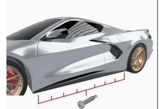
(1) Align splitter w/ rocker panel & proceed to install side splitter using self-drilling screws or hardware of your preference
