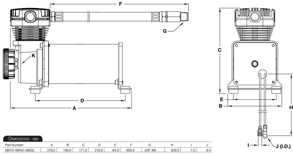
\* All measurements in millimeters, unless otherwise noted.
