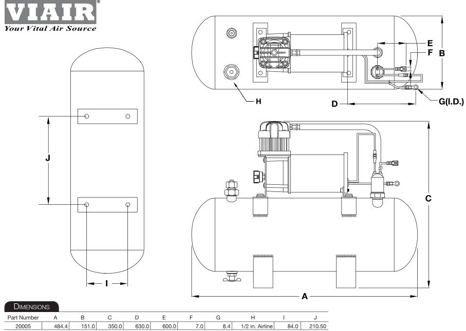
$^{\star}$  All measurements in millimeters, unless otherwise noted, +/- 1mm.  $^{\star\star}$  All fittings are NPT, unless otherwise noted.
