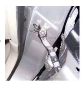
**3**) Remove Fender. Remove all plastic clips around the inner fender.
