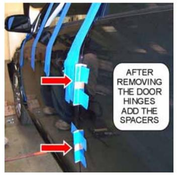
9) Install new hinge in place making sure it is flat against all contact surface, insert new bolts on firewall side and factory bolts on door side. Once the new vertical door hinge is secure remove the painter's tape. Hint\*(When locking hinge in place tighten bolts to door first then firewall bolts second)
