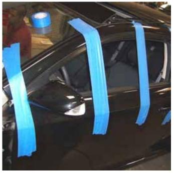
7) Close door and use painters tape to secure the door in preparation for factory hinge removal.
