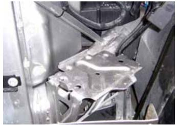
**4)** Remove the door catch: Open the door and remove bolts from the body and from the door. Push the door catch inside the door.
