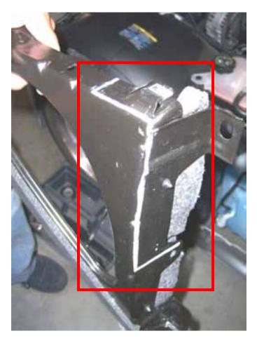
Remove the bolts holding the windshield fluid reservoir and the PCM assembly. Cut the bracket as shown. Drill and tap new hole to secure the assembly and use zip ties to secure the PCM
