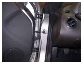
**5)** You will need to modify the wire layout: Remove the factory wire case and use wire loom to protect the exposed wires. As shown
