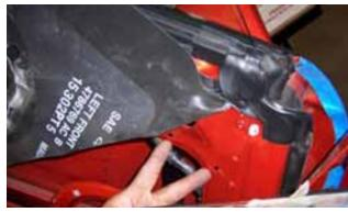
You will have to extend the wires going to the mirrors. Use the included wires.
