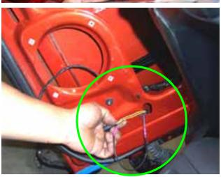
After the wires have been extended use zip ties to secure the wires to the original holes where the plug was before.
