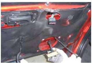
After removing the door catch pull back on the covering film and remove (2) plastic wire clips this will give you extra wire slack.
