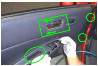
To gain access to the door catch you will have to remove the speaker.
