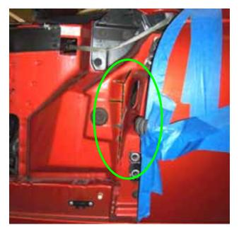
Use a hammer the bend the left side first and then the right side so that they form a flat surface and layer one on top of the other.
