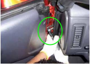
**5)** Remove the door panel: Remove the (3) screws securing the door panel, to remove the door handle cover you will have to carefully push in and slide it towards the back of the door.
