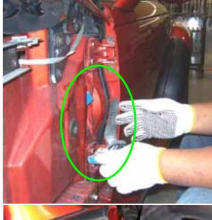
**4)** Remove the door catch: Open the door and remove the bolts securing it to the body and door, then push it inside the door we'll remove it later.
