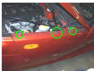
Before removing the fender make sure to disconnect the side marker wire harness.
