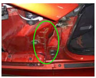
After achieving the flat surface use a rust preventing agent we used 3m window-weld ribbon sealer, to protect the exposed metal.
