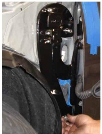
Hint\* Tighten the bolts on the door first and then install the bolts on the body.
