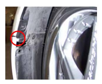
Now pull on the bumper and remove the remaining bolts securing the fender to the bumper and to the body.
