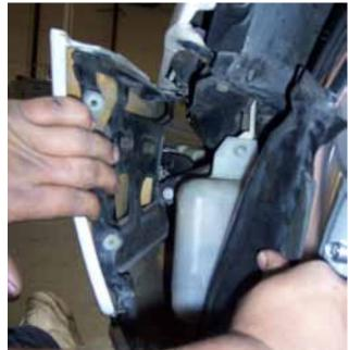
Remove the (3) 10mm bolts at the bottom of the door securing the fender to the chassis.
