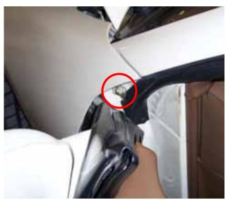
Remove all the bolts located at the top of the fender.
