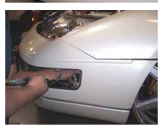
Remove all the fasteners around the wheel well.
