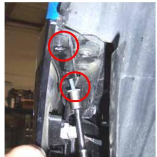
Now pull on the bumper this will allow you to remove (2) 10mm bolts securing the fender to the body.
