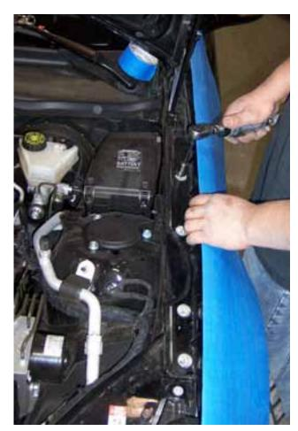
**3)** Open the door and remove (1) screw from the bottom hinge. Close door and use painter's tape to secure the door in preparation for factory hinge removal.
