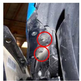
Use a Phillip's screwdriver to remove the (2) screws from the bottom of the skirt.
