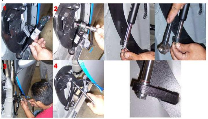
Hint\* (You will need a helper to raise the door). (Slip the spherical rod mount into the spherical ball bearing. Using a 1/4 Allen wrench, tighten the screw into the swing arm. After the shock is installed secure it by installing the pin in the bottom shock end.)
