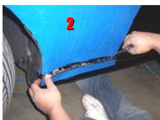
Pull on the wheel well to gain access to (2) 10mm bolts that secure the fender to the body. The bolts are in a bracket located next to the factory hinges, you will need to use an extension to reach them.
