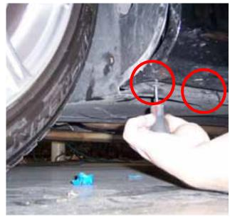
Open the door and remove the foot guard (PIC 1) and use the fork to **CAREFULLY** undue the first (2) plastic clips on the skirt (PIC 2).
