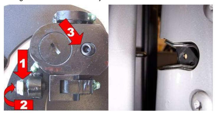
Hint\*(leave #1 nut loose until shock is installed Allen set screw will have to be re-adjusted after shock is installed.
