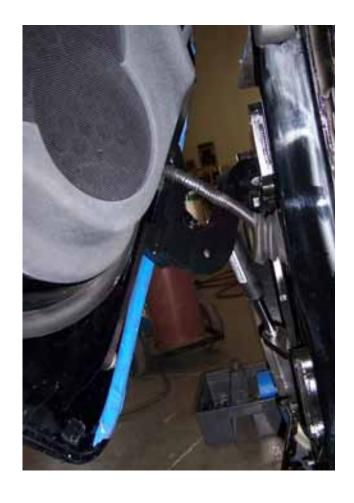
**10)** Cut the inner lip of your fender to make room for the new Vertical Doors hinge. Note: After you have cut the fender use a sander or grinder and take out any sharp edges, use black door trim to give it a finish look.
