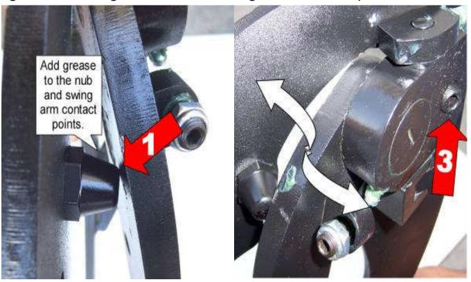
Hint\* (Fine tune the Allen set screw (#2) to realigned sticker with door. After the door is aligned, test door by opening and closing, lifting and lowering door several times.
