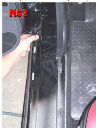
Close the door and use the fork to **CAREFULLY** pull on the skit to gain access to (2) 10mm bolts securing the fender to the body.
