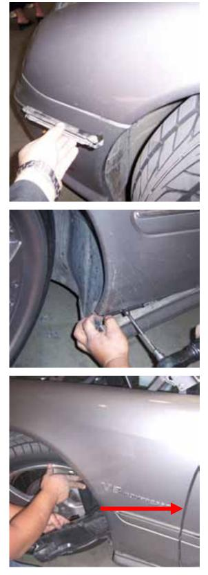
Remove (2), plastic covers (one on top and one on bottom) and use a 10mm socket to remove the bolts securing the fender to the hinge assembly.
