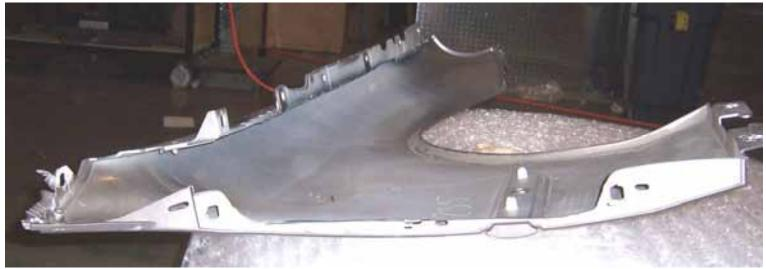
You will have to cut the inner lip of the fender as showed. Use a grinder to remove any sharp edges and black door trim to give it a finish look.
