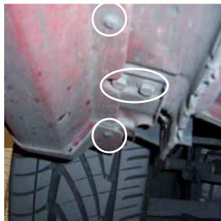
Open the door and remove one 10mm screw located at the bottom of the windshield pillar.
