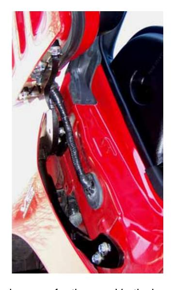
**12)** Cut the inner lip of your fender to make room for the new Vertical Doors hinge. Note: After you have cut the fender use a sander or grinder and take out any sharp edges, use black door trim to give it a finish look.
