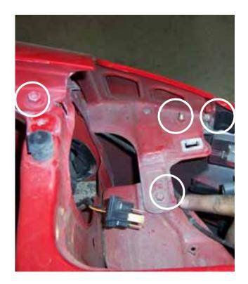
On the back of the wheel well (closest to the door) remove (2) Phillips screw located under the skirt. This will allow you to pull on it and remove (2) 10mm bolts securing the fender to the body.
