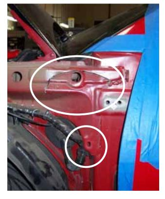
After bending the notch on the apron you will be able to install the new VDI system.
