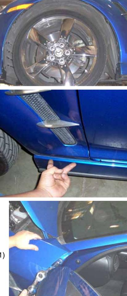
After you have removed all fasteners from wheel well remove (1) 10mm bolts from the bottom of the skirt, this will allow you to pull on it to access (2) 10mm bolts securing the fender to the body.
