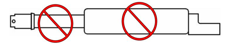
WARNING! THE USE OF ANY TYPE PLYERS, PAINT OR FOREING MATERIALS ON THE SHOCK'S BODY OR SHAFT WILL VOID THE WARRANTY.
