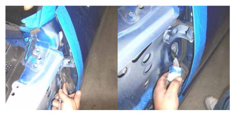
You will need more wire slack with the door panel off, use a knife or any other type of cutter and cut (2) wire fasteners, so that you are able to pull on the wire.
