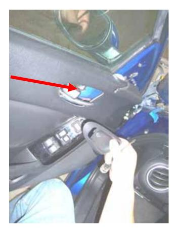
Use the fork to remove the plastic control panel and a Phillip's screw driver to remove the screws.
