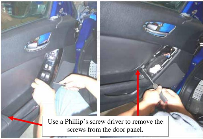
Now carefully remove the door panel and disconnect the (2) light harnesses.
