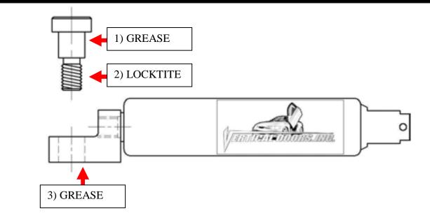
\*IMPORTANT STEP: DO NOT SKIP THIS STEP. THIS STEP IS CRUCIAL IN YOUR INSTALLATION PROCESS, IF THIS STEP IS NOT COMPLETED WHEN INSTALLING THE VERTICAL DOOR KIT; ALL WARRANTIES ARE VOIDED, AND MAY CAUSE FUTURE PROBLEMS WITH YOUR VERTICAL DOOR SYSTEM. 1<sup>ST</sup>, make sure you put grease on the body of shoulder bolt where the arrow is pointing.
