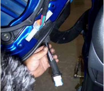
Cut the factory wire loom in half and add aftermarket wire loom to protect exposed wires. 6) Close the door and use painter's tape to secure the door to the body in preparation for factory hinge removal.
