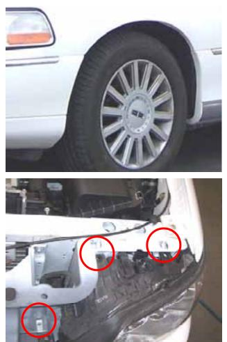
Note: one of the bolts securing the fender to the body goes through the body you will need to remove the foot trim and the kick plate to gain access to the 10mm nut securing the fender.
