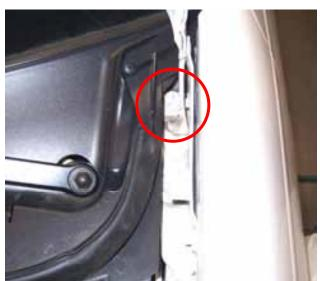
After removing the door panel, pull on the bottom of the protective film and undue (3) plastic wire clips as shown.
