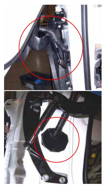
**12)** Cut the inner lip of your fender to make room for the new Vertical Doors hinge. Note: After you have cut the fender use a sander or grinder and make sure the surface is completely flat.
