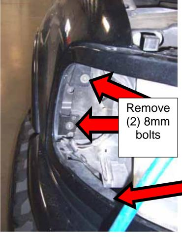
(Figure 2) Lift up on the windshield plastic cover and remove (1) 8mm bolt. Remove the rest of the 8mm bolts from the top lip of the fender.
