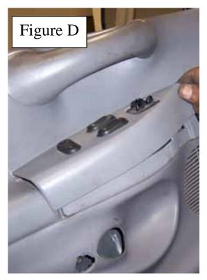
Unplug the wire harness (figure E) and use the fork to remove the plastic clips in the front (figure F) and back (figure G) holding the door panel in place after you have remove the clips pull on the door panel and unplug the small light (figure H) on the back of the door panel. At this time you should be able to remove the door panel.
