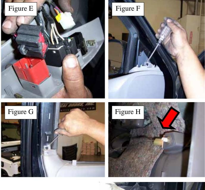
6) Modify wire layout: You will need more wire slack in order for the Vertical Doors Inc. system to open all the way up. Use the fork to remove (3) plastic clips to gain more wire slack from the door.
