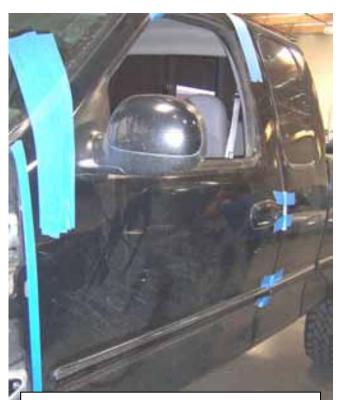
Add the spacers after you have removed the factory hinge.
