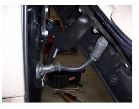
**12)** Cut the inner lip of your fender to make room for the new Vertical Doors hinge. Note: After you have cut the fender use a sander or grinder and make sure the surface is completely flat.
