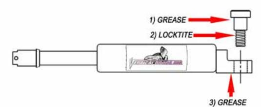
\*IMPORTANT STEP: DO NOT SKIP THIS STEP. THIS STEP IS CRUCIAL IN YOUR INSTALLATION PROCESS, IF THIS STEP IS NOT COMPLETED WHEN INSTALLING THE VERTICAL DOOR KIT; ALL WARRANTIES ARE VOIDED, AND MAY CAUSE FUTURE PROBLEMS WITH YOUR VERTICAL DOOR SYSTEM.
