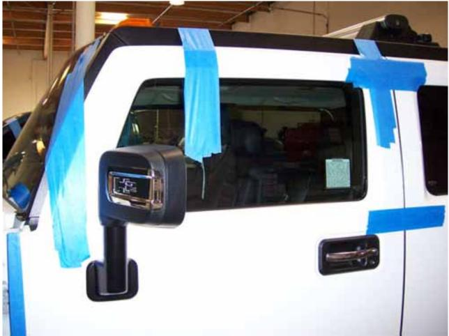
5) Prepare area for the new Vertical Doors Inc. system. Remove the factory door hinges, tape up and cut the bump where the new Vertical Doors Inc system will be placed.
