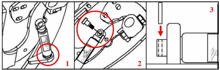
Hint\* (You will need a helper to raise the door). (Slip the spherical rod mount into the spherical ball bearing (1). Using a 1/4 Allen wrench, tighten the screw into the swing arm (2). After the shock is installed secure it by installing the pin in the bottom shock end (3).
