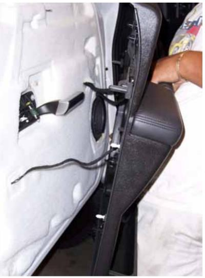
4) Tape up the door. Use blue painter's tape to secure the door to the body.
