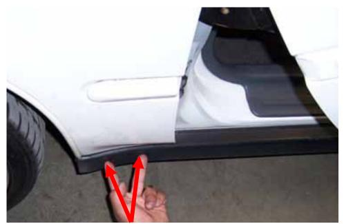
Remove (2) 8mm bolts from the bottom of the fender by the door.
