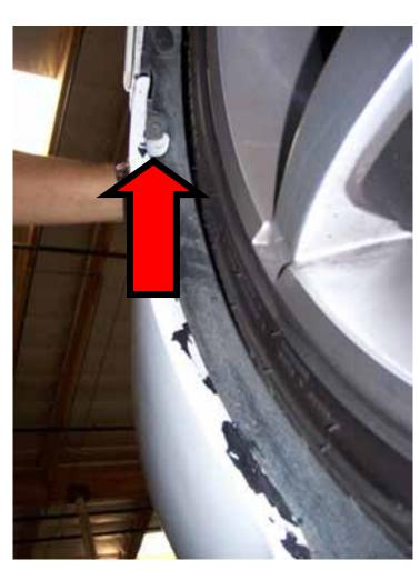
Remove (1) 12mm bolt to loosen the bumper.
