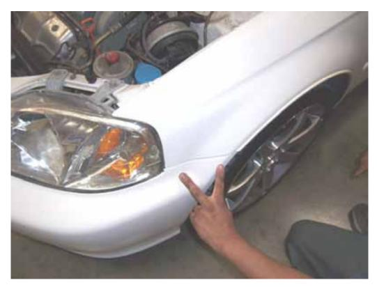
Remove (3) 8mm bolts form the top of the fender.
