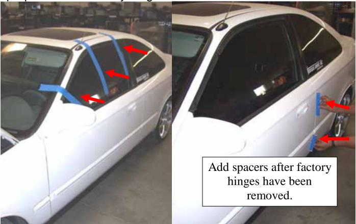
Use a 13mm socket to remove the factory hinges.
