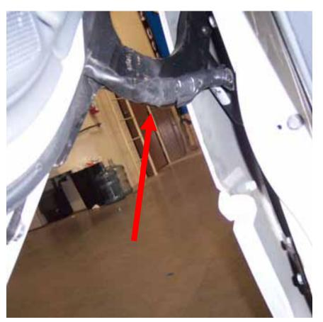
11) Cut the inner lip of your fender to make room for the new Vertical Doors hinge. Note: After you have cut the fender use a sander or grinder and make sure the surface is completely flat.
