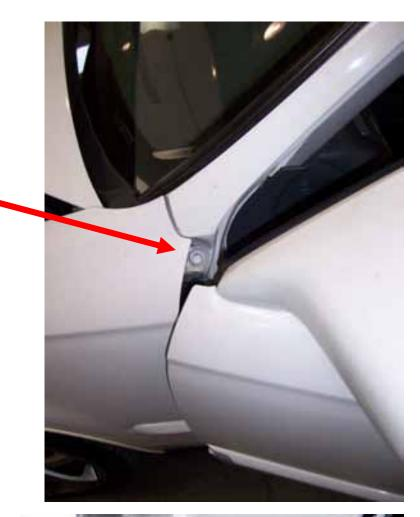
3) Remove the door catch: Open the door and remove (1) 10mm bolt from the body and (2) 10mm from the door. Push the door catch inside the door.
