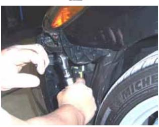
Remove the bolts securing the fender to the chassis at the bottom of the door.
