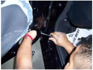
**5)** Close door and use painter's tape to secure the door in preparation for factory hinge removal.
