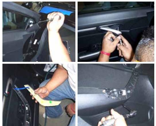
After removing the door panel, remove the speaker. And the wire clip closest to the speaker this will give the necessary wire slack for the new VDI kit to open fully and also the clearance to remove the door catch.
