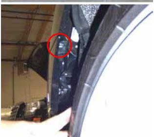
After removing the bolt securing the fender to the bumper, pull on the bumper to gain access to the bolts securing the fender to the body.
