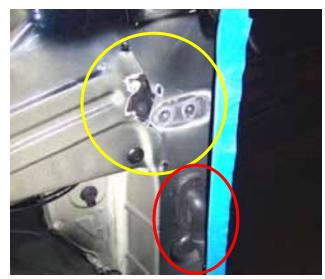
Note: you will have to pull the factory wire boot cut it in half and flip it up side down to gain extra wire slack.
