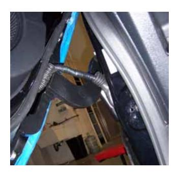
**11)** Cut the inner lip of your fender to make room for the new Vertical Doors hinge. Note: After you have cut the fender use a sander or grinder and make sure the surface is completely flat.
