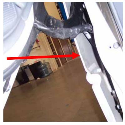
The fender should look like the picture above when you are done cutting it. 12) Lift the door and Replace the fender by reversing step 2.
