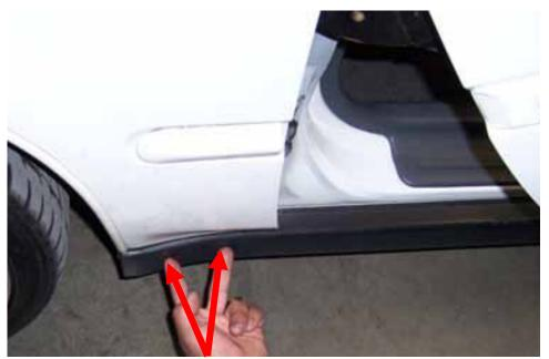
Remove (2) 8mm bolts from the bottom of the fender by the door.
