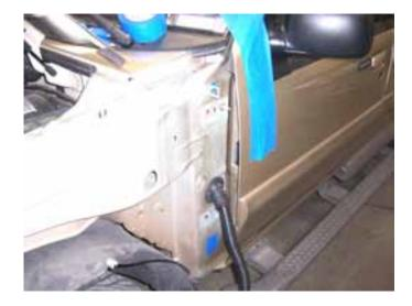
After doing that remove the factory door hinges from the body and the door.
