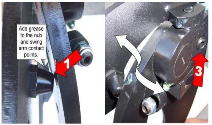
Hint\* (Fine tune the Allen set screw (#2) to realigned sticker with door. After the door is aligned, test door by opening and closing, lifting and lowering door several times.
