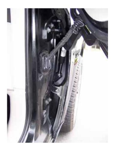
**11)** Cut the inner lip of your fender to make room for the new Vertical Doors Inc. system. Note: After you have cut the fender use a sander or grinder and take out any sharp edges, use black door trim to give it a finish look.
