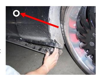
Remove all the fasteners from the top of the fender.
