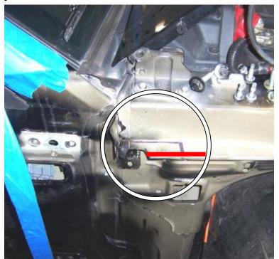
After cutting the notch on the apron lip you will be able to install the new VDI system.
