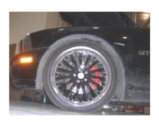
With the wheel well fasteners removed, use the fork to pull on the wheel well to gain access to (2) 10mm nuts this will allow you to pull on the bumper.
