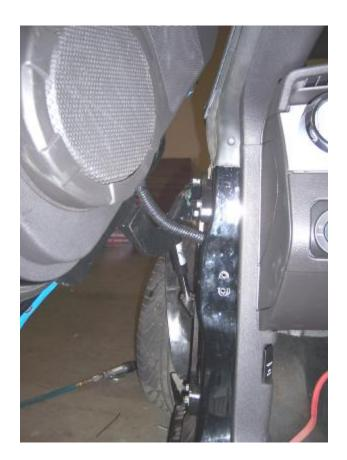
**12)** Cut the inner lip of your fender to make room for the new Vertical Doors hinge. Note: After you have cut the fender use a sander or grinder and take out any sharp edges, use black door trim to give it a finish look.
