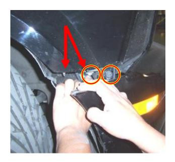
On the back of the wheel well (closest to the door) pull down on the skirt this will give you access to (2) 10mm bolts securing the fender to the chassis. Pull on the wheel well and use a socket with an extension to remove (1) 10mm bolt securing the fender to the body, located by the factory hinge.
