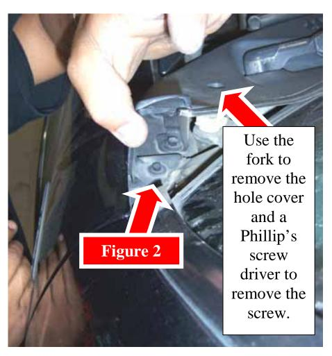
Remove (4) 7/32 screws from the wheel well and any other fasteners holding it.
