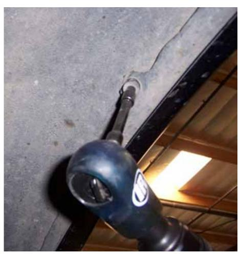
To remove the remaining (2) 8mm bolts (figure A), you will have to pull on the wheel well and remove the plastic or foam that cover the factory hinges (figure B). After removing the foam you will be able to remove the (2) 8mm bolts that are located by the factory hinges.
