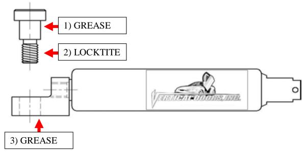
\*IMPORTANT STEP: DO NOT SKIP THIS STEP. THIS STEP IS CRUCIAL IN YOUR INSTALLATION PROCESS, IF THIS STEP IS NOT COMPLETED WHEN INSTALLING THE VERTICAL DOOR KIT; ALL WARRANTIES ARE VOIDED, AND MAY CAUSE FUTURE PROBLEMS WITH YOUR VERTICAL DOOR SYSTEM.
