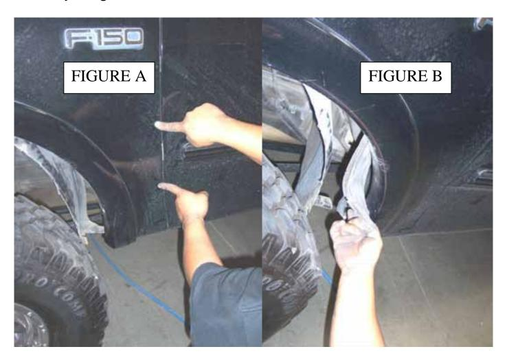
At this point use the fork on the front by the head light to help you remove the fender.
