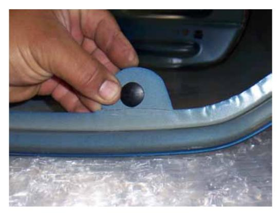
11) Cut one of the fender clip holders to make room for the new Vertical Doors hinge. Note: After you have cut the fender use a sander or grinder and make sure the surface is completely flat.
