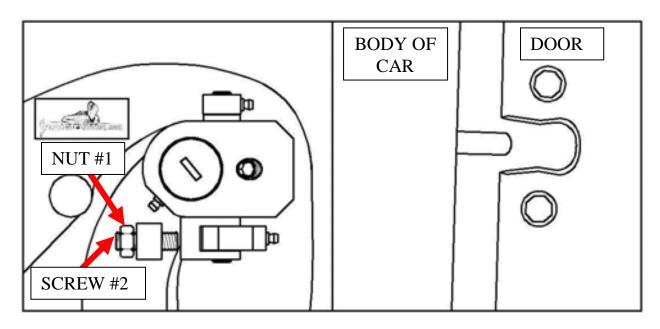
Hint\*(leave #1 nut loose until shock is installed Allen set screw will have to be re-adjusted after shock is installed.
