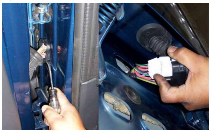
Open the door and use the fork to remove the factory wire boot, unplug the wire harness and push it back in the hole and the other side inside the door.
