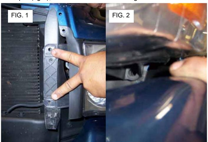
Now disconnect all (3) wire harnesses from the head light, and remove the head light and signal lights.
