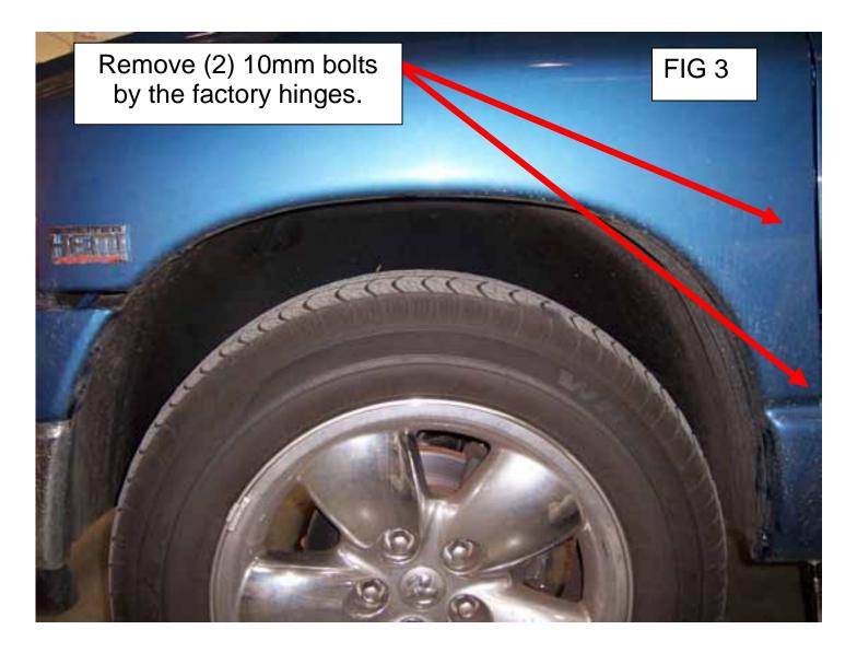
To remove the bolts on (fig 3) you will have to remove all the fasteners on the wheel well then pull on the wheel well closest to the door to gain access to the (2) bolts.
