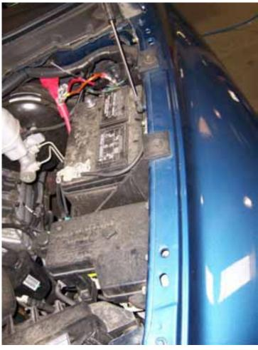
Remove (4) 10mm bolts on top of the fender and (2) 13mm bolts that hold the battery.
