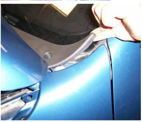
The last 10mm bolt is located under the windshield plastic cover.
