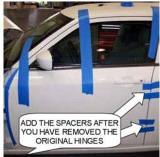
6) After you have removed the original door hinges, install the New Vertical Doors Inc. System. Make sure all mounting surfaces are flat.
