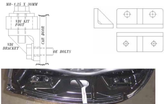
6) Installing the brackets to the body, as shown.
