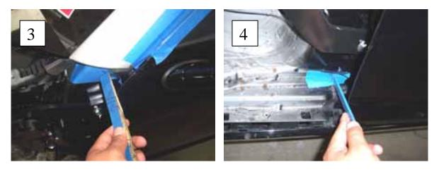
After marking the door and disconnecting the wire harness remove the door.
