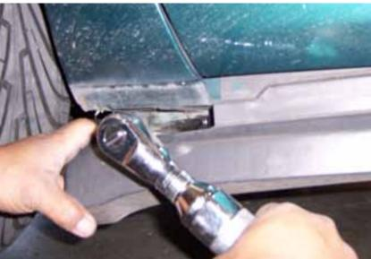
Use the headlight hole to gain access to (2) 11mm bolts securing the fender to the bumper, this will allow you to pull on the bumper to remove (1) 10mm bolt securing the fender to the body.
