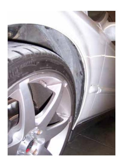
On the skirt, remove one plastic clip this will release the front end of the skirt enough to pull on it, to gain access to (2) 10mm bolts.
