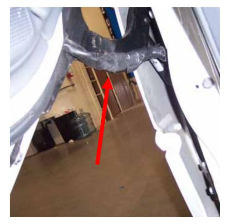
12) Cut the inner lip of your fender to make room for the new Vertical Doors hinge. Note: After you have cut the fender use a sander or grinder and make sure the surface is completely flat.
