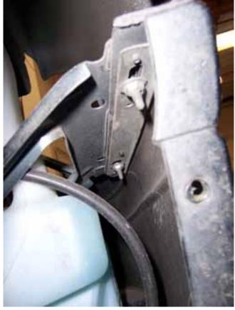
Pull on the wheel well and remove the plastic or foam cover located by the factory hinges. Use a 10mm socket to remove (1) 10mm bolt.
