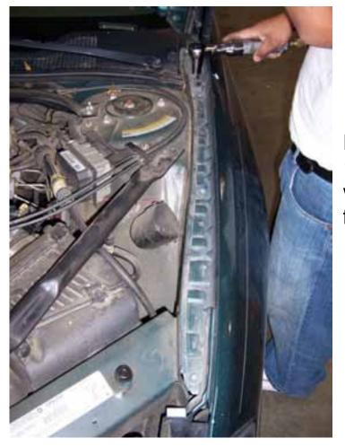
Remove (3) 10mm bolts and (2) 13mm bolts. At this point you will be able to remove the fender.
