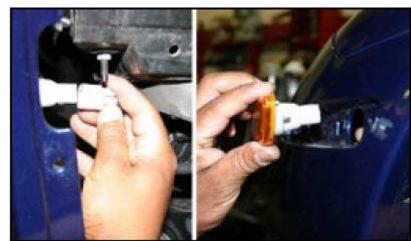
Look inside inner fender and above where the turn signal was, unscrew three bolts.
