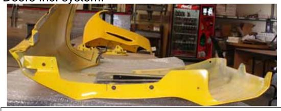
Use a power cutter and grinder to cut and take any sharp edges off. Use black door trim or touch it up with paint to give it a finish look.
