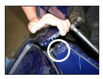
Pull upward on front bumper cover as shown and remove screw with T15 Torx wrench.
