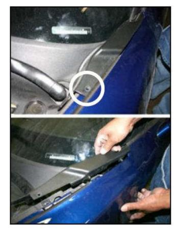
Starting from the front of car, lift off fender and locate the only remaining 7mm screw that is attaching the fender to the rest of the body. The screw is located near the stock door hinge.
