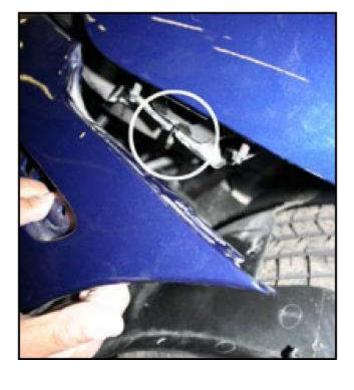
Using 7mm socket, remove (4) screws from front bumper cover underneath hood area.
