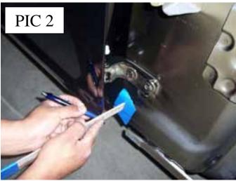
5) After making sure you have all the marks you need in case the door moves during installation, you can remove the factory door hinges. After installing the new VDI kit you should be able to raise the doors and start the fine tuning you're your new VDI kit.
