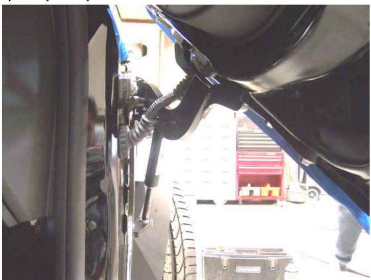
In order to be able to open and raise the door, cut the factory wire boot in half and add wire loom to protect exposed wires as shown note the routing of the wires.
