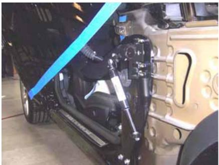
Note: wire loom will have to be cut in half, use provided wire loom to protect the exposed wires.
