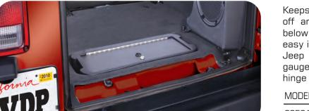
Keeps valuables safe and secure when top is off and doors unlocked. Discreetly hidden below rear cargo floor carpet. Quick and easy installation securely bolting to existing Jeep body vault. Crafted design with 16 gauge steel lid and stainless steel piano hinge makes it impossible to pry open.
