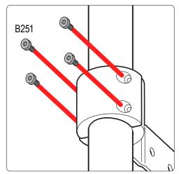
Do not completely tighten bolts so adjustments can be made later on.
