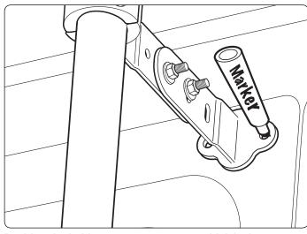
Position the ladder mounts onto your vehicle's door.
