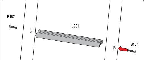
Do not completely tighten bolts so adjustments can be made later on.
