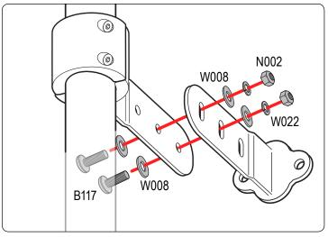
Depending on your curve of your vehicle you can use hole combinations to create different angles. Have 2 bolts per mount
