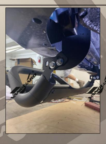
5. Install the fixing screws.
