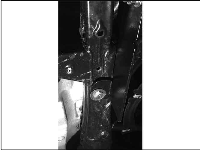
(Fig 4) Hold Bracket up to factory hex bolt to determine approximate area to cut out of splash guard. Mark location (left) and remove splash guard. Cut out both areas as required to clear Brackets (right). Areas marked and cut pictured for example only
