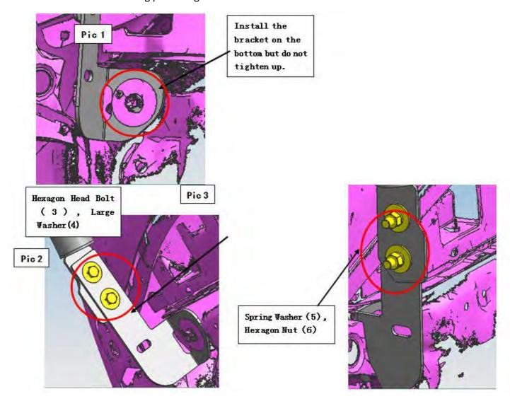
Step 3: Check if all hard ware are installed and after adjusting all brackets, tighten up all hardware and complete the installation.
