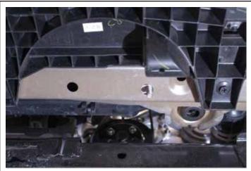
Insert (2) 5/16" Bolt Plates into the outer holes on the lower radiator support. Hold up the brace to verify fitment.
