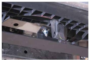
Attach the brace with (1) 5/16" Flat Washer and (1) Lock Washer per side.
