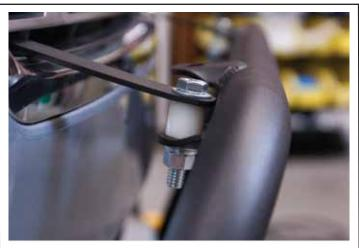
Attach the Light Bar as shown with (1) 3/8" x 1.75" Hex Bolt, (1) Flat Washer, (1) 3/4" Nylon Spacer, (1) Flat Washer, (1) Lock Washer, and (1) Hex Nut per side.
